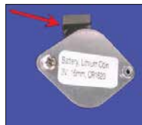
Remove Battery Insulating Tab.
