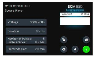
Voltage, Duration, Number of Pulses, Pulse Interval, and Electrode Gap may be modified by tapping on the gray icons for each. Green Accept icon may be tapped to proceed to Run Protocol screen.
