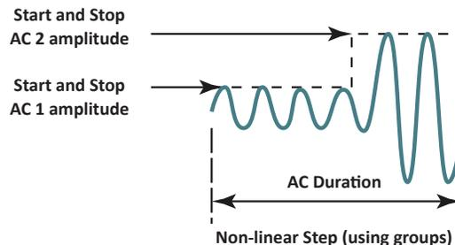
Figure 19: AC Sine Wave Amplitude Functions
