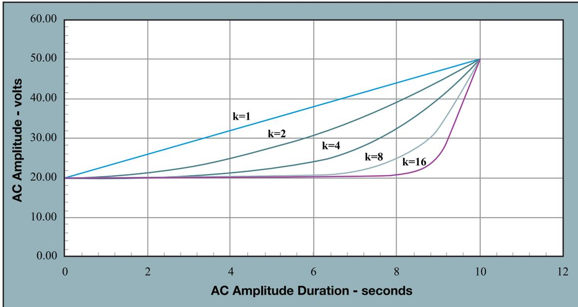
Figure 20: Ramp k Factor in Non-Linear Sine Wave Amplitude
